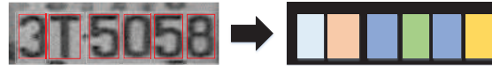
Fig. 3. Illustration of box-level label for a license plate image. The sample is from the AOLP dataset. Here different colors denote different character classes. The pixels not belonging to any character box are labeled as the background class (black). Best viewed in color
