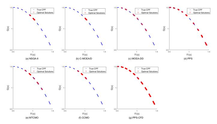
Fig. 3. Results achieved by each algorithms on LIRCMOP3. Blue solid lines represent CPF, red dots represent feasible and non-dominated solutions, and white areas represent infeasible regions.
