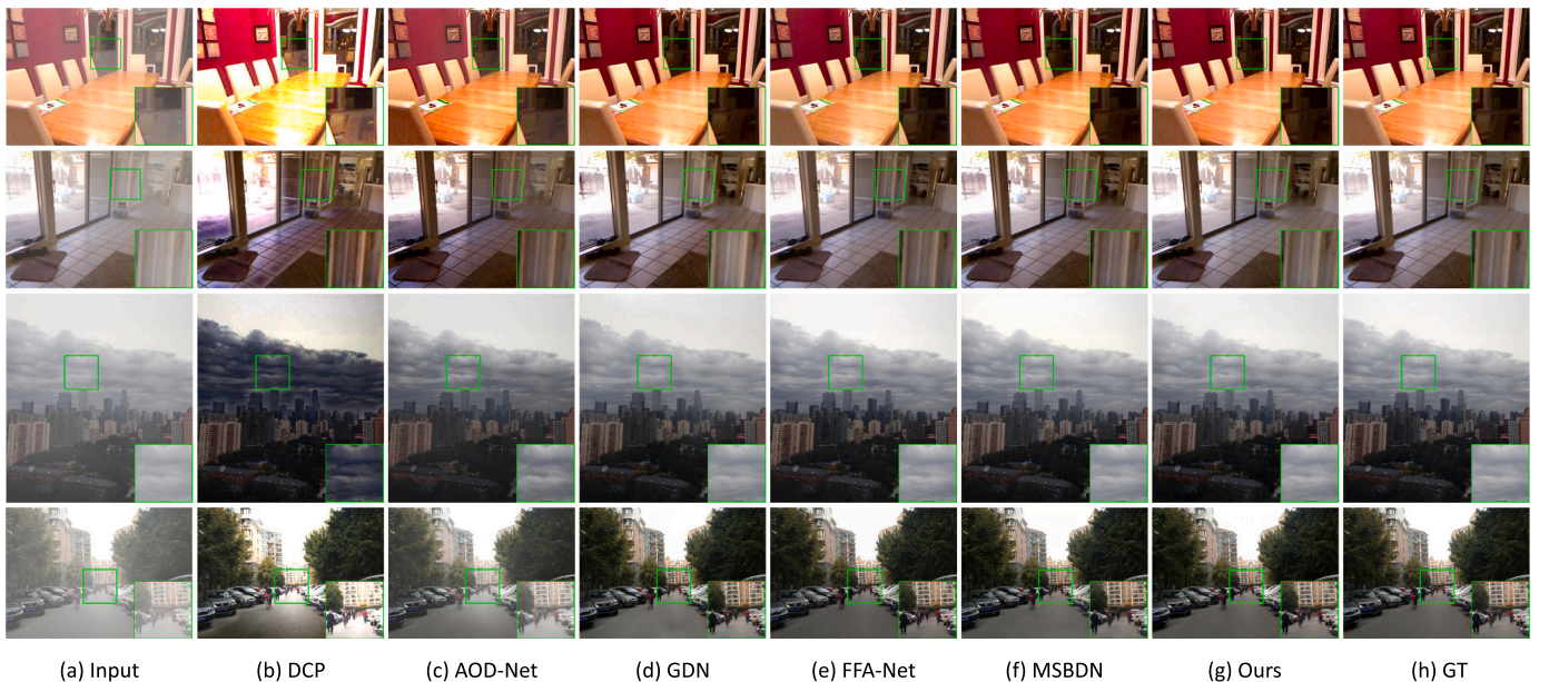
Fig. 8. Comparison of dehazing results on SOTS (Indoor) and SOTS (Outdoor) datasets. The first two rows of hazy images are from SOTS (Indoor), and the last two rows are from SOTS (Outdoor).
