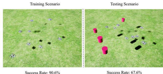
Fig. 1. **Illustration on the influence of spurious correlations.** Due to the presence of spurious correlations, deep reinforcement learning algorithms have a tendency to memorize solutions of seen obstacles in the training scenario, thereby achieving high training rewards with a brittle policy that will not generalize to unseen obstacles in the testing scenario.
